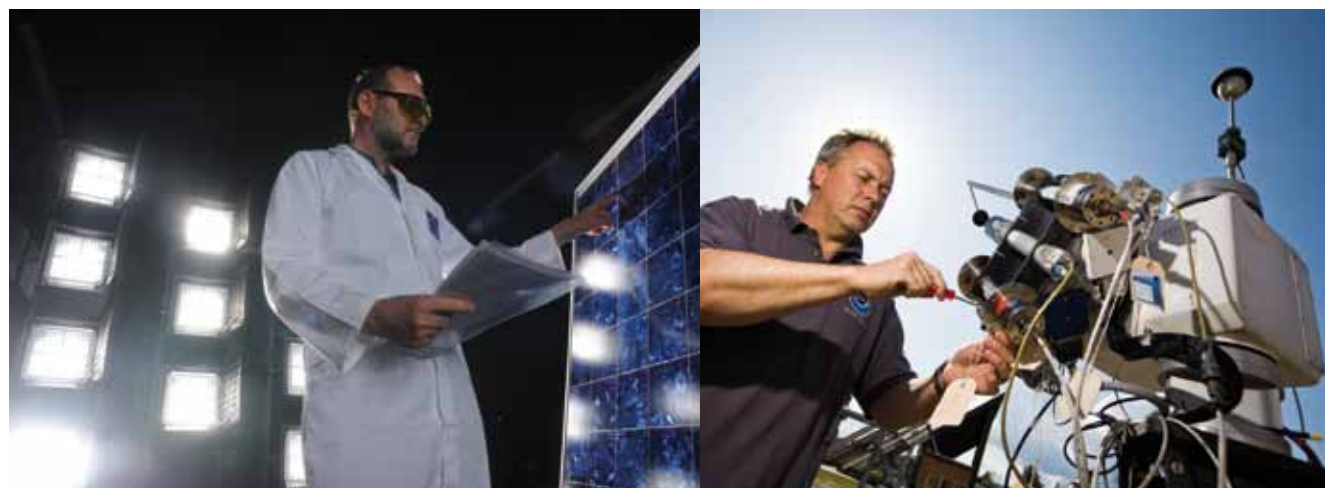
ESTI's new large-area steady state simulator opens a range of possibilities for studying the electrical performance of new module technologies with long response times.
